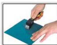
step 1: make grid cutting on surface
