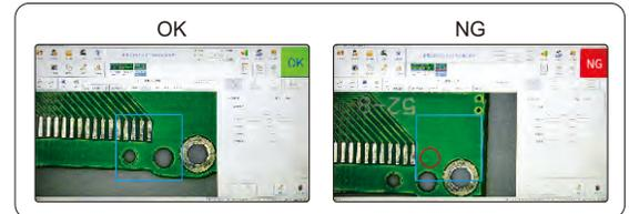
select the area and specify the target, the camera will automatically detect the presence or absence of the target.
