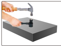
hammer impact to apply test force
