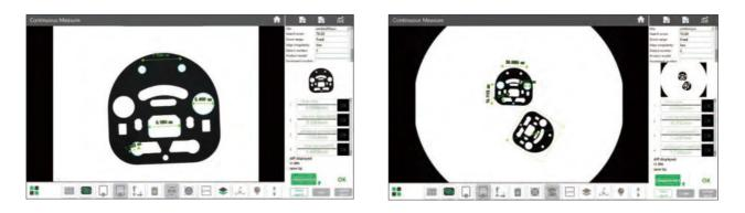
• Measuring result can be stored automatically. OK items and NG items can be counted automatically.
